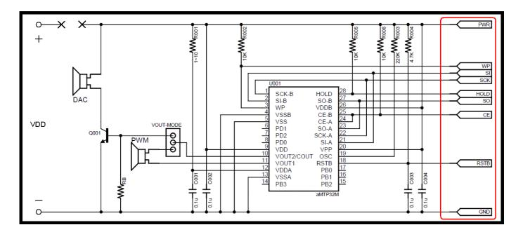
• Warning: aSPI28W PWR pin will offer power to circuit. So before connecting to aSPI28W, you must remove any other power source and device which may input signal to circuit.
