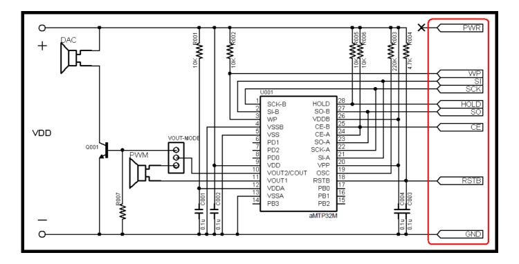
• User provide supply VDD, VDD need between 3.3V and 3.6V.
