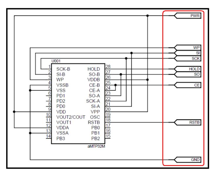
• Warning: aSPI28W PWR pin will offer power to circuit. So before connecting to aSPI28W, you must remove any other power source and device which may input signal to circuit.
