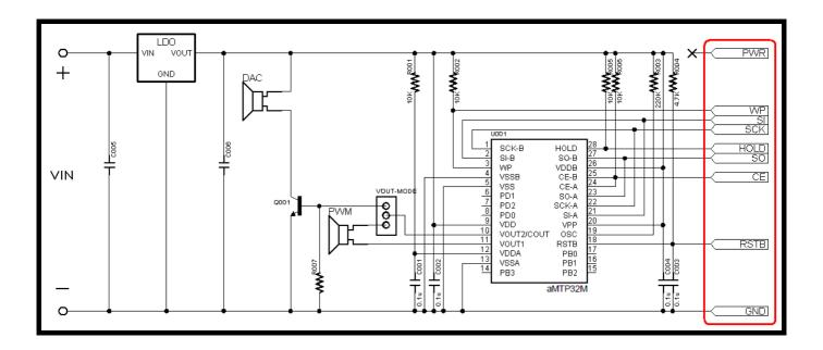
• User provide supply VDD, VDD need between 3.3V and 3.6V.
